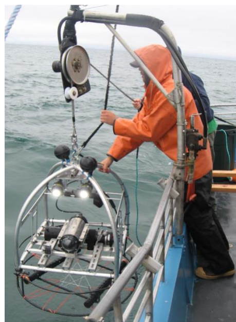
Image: Deploying/retrieving a video lander. Source: ODFW Information Report 2019-20, p. 41
