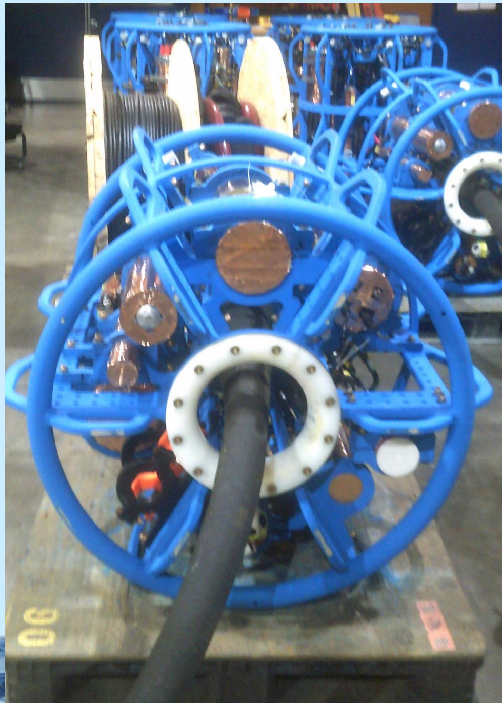
Application of diaper cream on acoustic transducers to prevent biofouling
