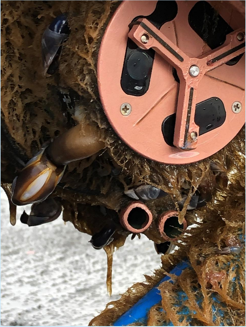
Copper and wipers prevent sensor biofouling
