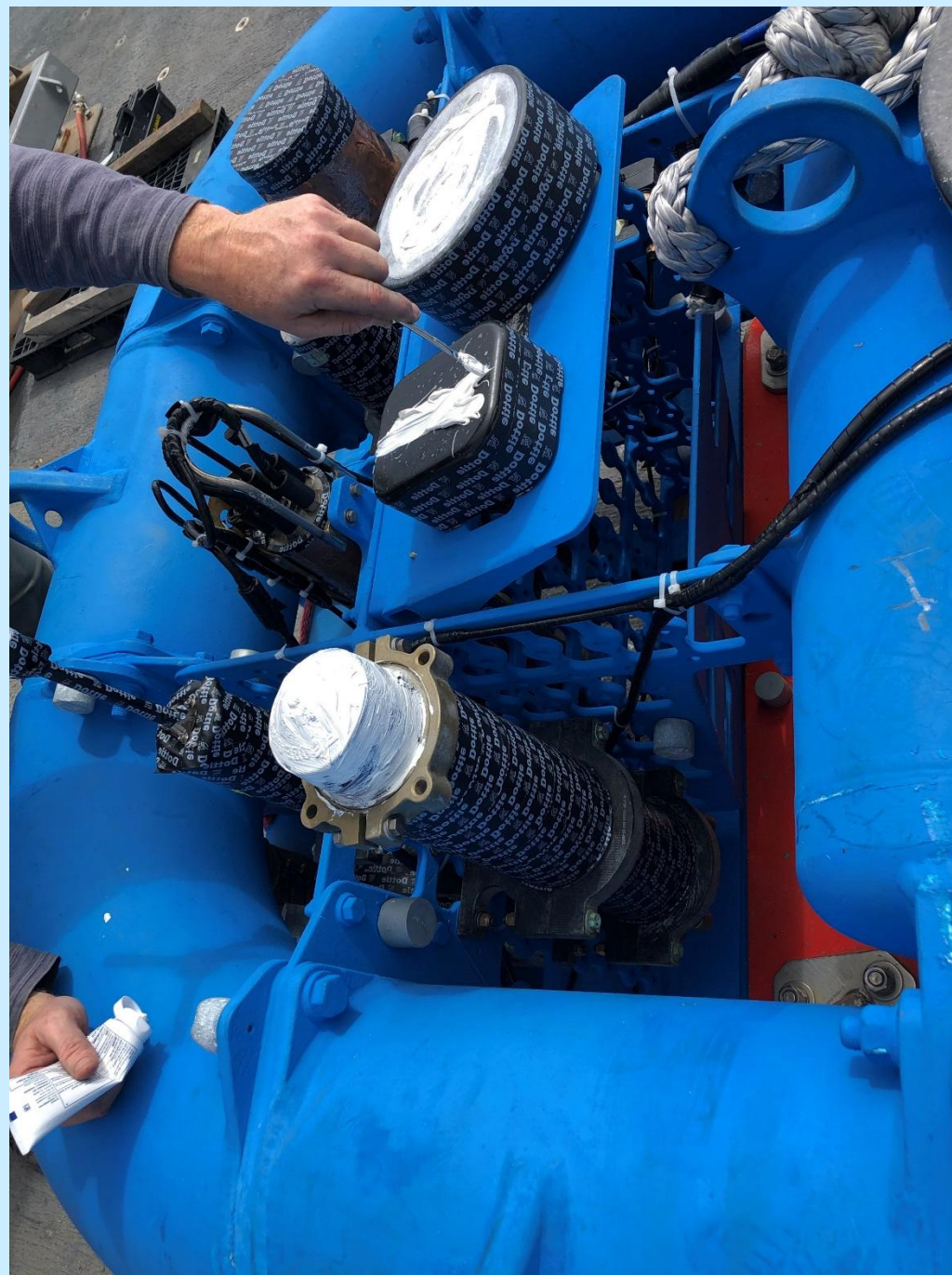
Application of diaper cream on acoustic transducers to prevent biofouling
