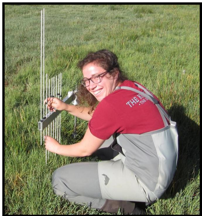
*A South Slough intern measuring the distance between the RSET and the marsh surface using pins.*
