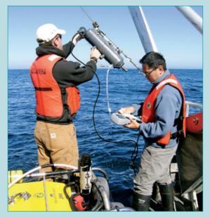
PISCO scientists measuring oxygen content in seawater from a sampling bottle that has been lowered to a precise depth. The ROV operated by ODFW appears in the lower left corner. *Photo: Jane Lubchenco*
