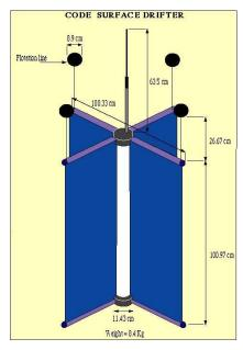
Four major components make up a drifter. These include a waterproof tubular body, sails, spherical floats, and a data collection/transmitter package. Use Google Earth to have students view or track drifters that have been deployed.
